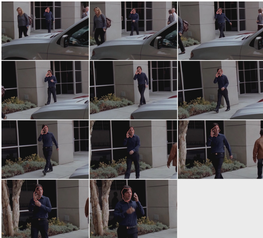
Figure 12: Tracking output of every 15 th frame of the face sequence (local tracking)
